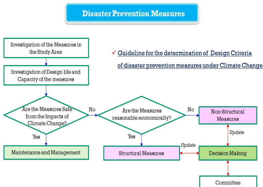
**Figure 2.** Decision making procedure for the application of future design criteria under the climate change
